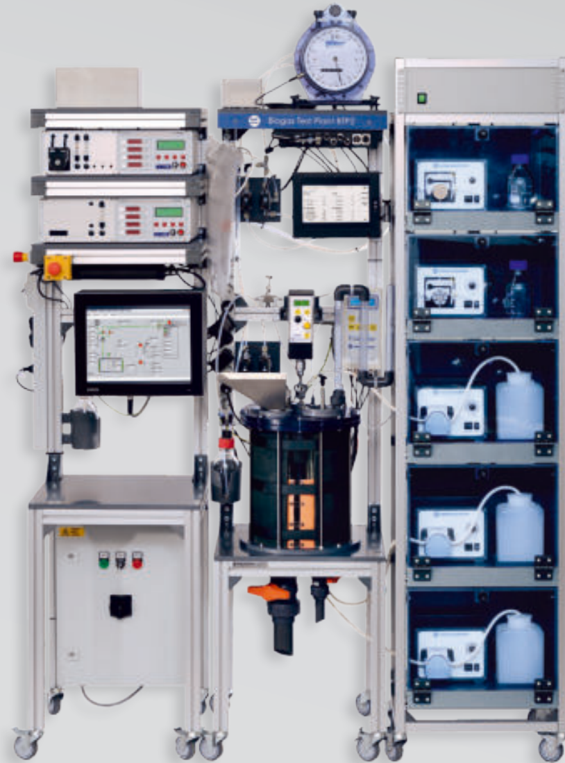
BTP2-control with pump modules
